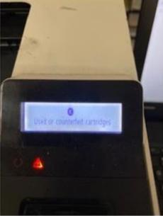
Once you press OK, the cartridge is good for the life of the toner, even if the printer is power cycled or the cartridge is taken out and shaken and reinstalled. It will continue to display the "ready" message below until a new toner is installed.
